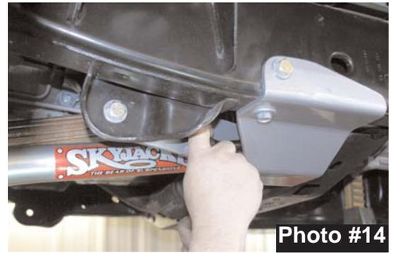
18. Locate new Skyjacker lower control arms. (Fronts are longer than the rear) Install the supplied poly bushings and sleeves. It is recommended to apply a thin coat of lithium grease to bushings and sleeves prior to installation. Be sure to install the 1/4" drive in zirk fittings. These are easily driven in with the use of a 1/4" socket. Install the supplied 1 1/4" Rod End and jam nut. Be sure to install the 14mm bolt inserts.
