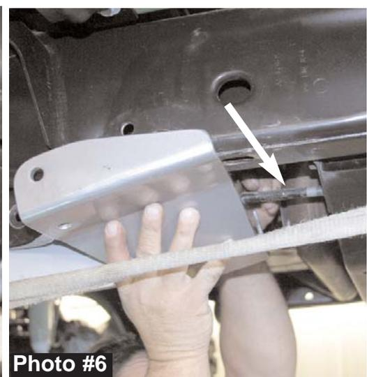
10. Install factory skid plate bolt that was removed in step #6. (See Photo #7).
